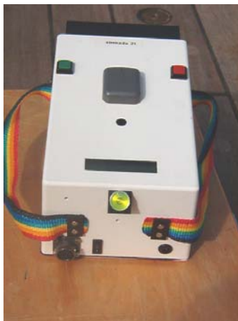
Figure 3: showing equipment used for solar light measurements: the Simbada-21 (left-hand side) and the Hyperspectral radiometer on the right ( reproduced from Brian Irwin's talk ).
