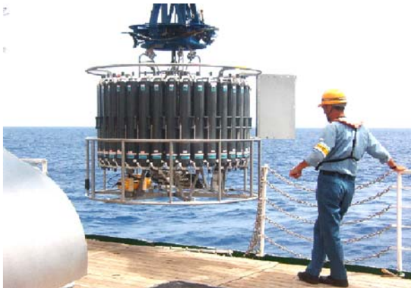
Figure 2: Showing the Conductivity Temperature Density (CTD) device. The CTD was used to collect water samples at pre-determined depths, for different analyses.
