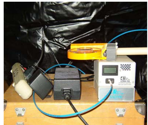
Figure 3: showing equipment used for solar light measurements: the Simbada-21 (left-hand side) and the Hyperspectral radiometer on the right ( reproduced from Brian Irwin's talk ).
